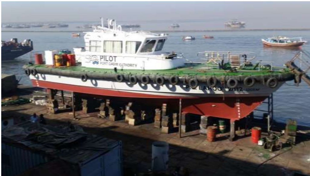
PQA Pilot Boat LAHOOT hoisted at south quay wall for repair work on propulsion system
